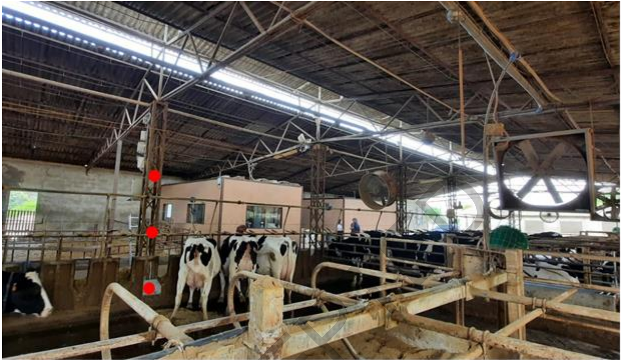
538 Figure 2. Indoor view of the barn, position of SLs in the vertical spots (i.e., red points), and box containing INNOVA 539 and Digitron sampling systems and air filters.
