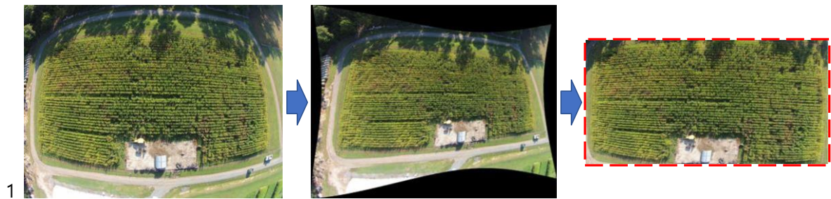
2 (a) Distorted image (b) Undistorted image (c) Bird's eye view and cropping
